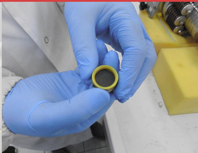
Detail of a new material sample during the insertion process inside the gas chambers of Real Life Tester.
